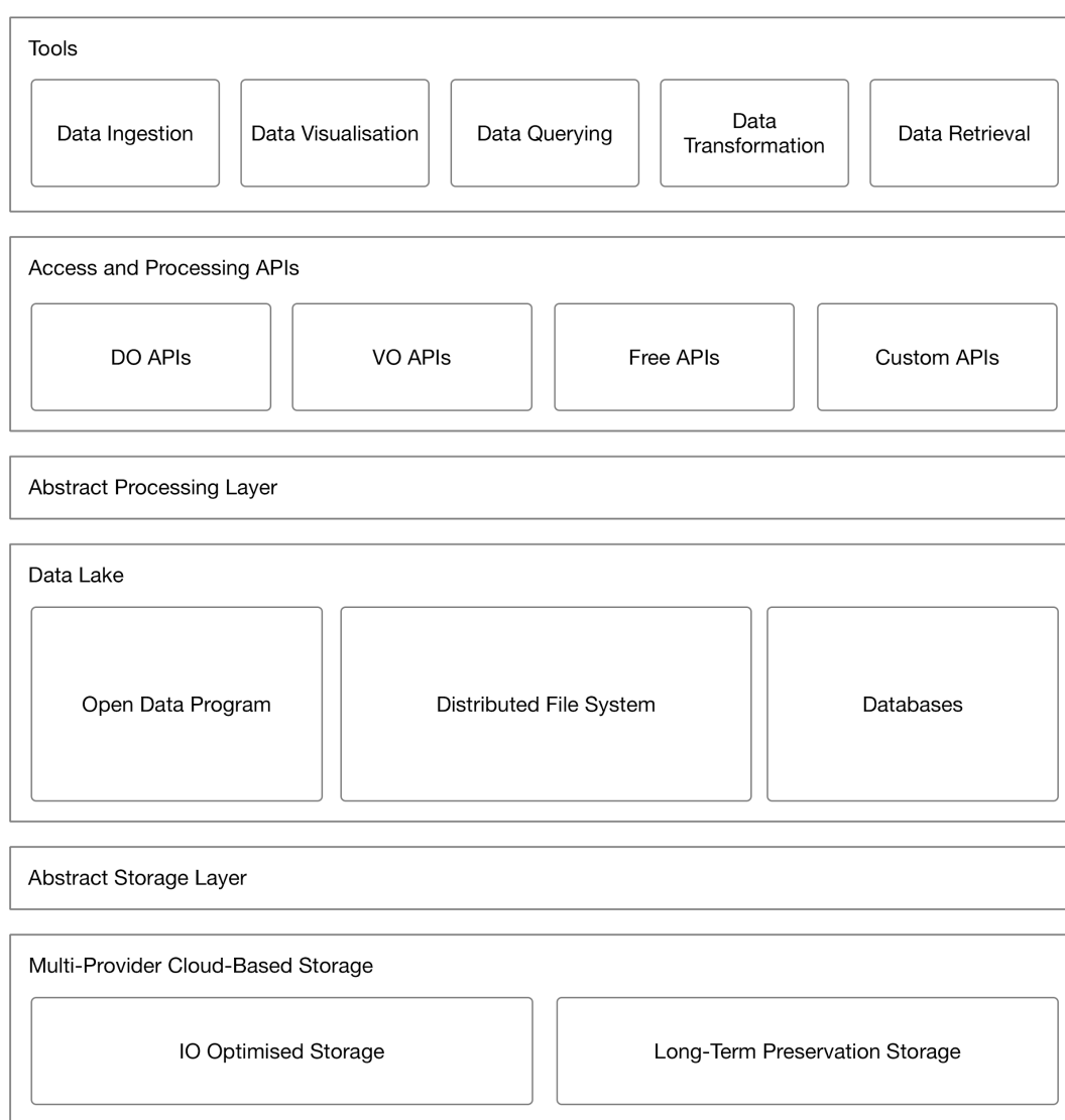
Figure 5: Layered View of the DO computing resource architecture.
